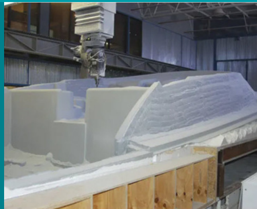
A FIVE AXIS MILLING MACHINE FORMS THE DECK PLUG FOR A 42' VIKING. IMAGE COURTESY: PMY
