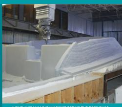
A FIVE AXIS MILLING MACHINE FORMS THE DECK PLUG FOR A 42' VIKING. IMAGE COURTESY: PMY
