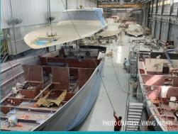
Viglass also builds many other large fiberglass structures, such as deckhouses, bridges, and fiberglass fuel tanks, as well countless small parts. Above: Shipwrights guide the deckhouse of a 68 forward on Line 1 from Viglass (left) into Mechanical (right), where it will be lowered onto its awaiting hull.
