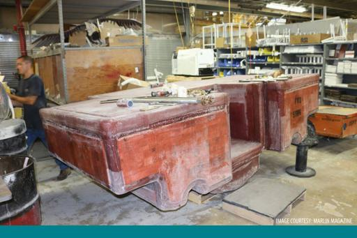
After the hull is molded, fiberglass encapsulated stringers, bulkheads, and egg crating are installed and bonded to the hull, adding strength, internal structure, and support.
