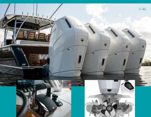
The Mercury 7.6-Litre V12 600-hp Verado remains static, and steering occurs underwater using a steerable gearcase which can pivot up to 45-degrees under joystick operation.
