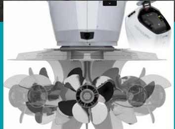
**The Mercury 7.6-Litre V12 600-hp Verado remains static, and steering occurs underwater using a steerable gearcase which can pivot up to 45-degrees under joystick operation.**
